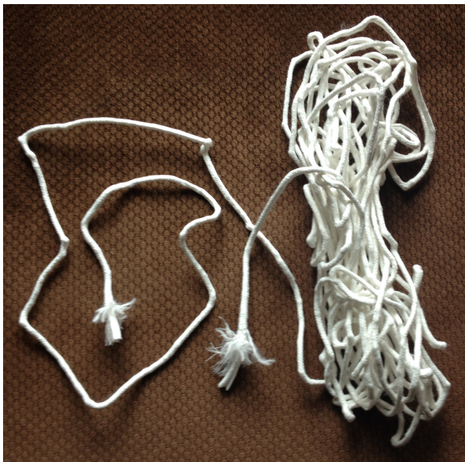
Figure 2. Rope used in the demonstration, showing kinks and frayed ends.
