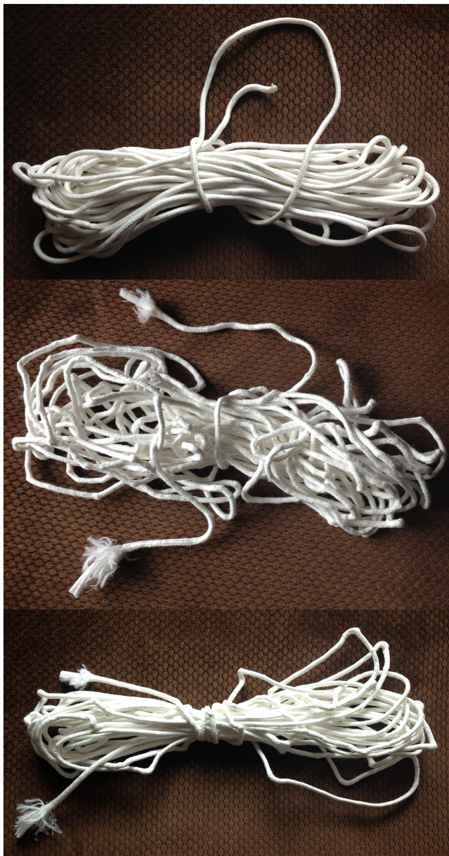
Figure 5 (bottom right). Second rope found the morning after the demonstration. Never used and still neatly wound, but stiff and showing the same elbow-type kinks and frayed ends as the demo rope.
